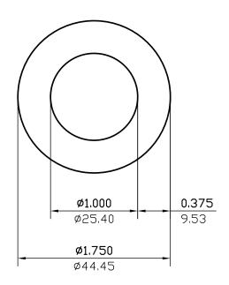
(AS SHOWN) WALL THICKNESS EXCEPT AS SHOWN DATE REV DESCRIPTION BY 03/10/23 REMOVED ALLOY JASON 1045.092 ın.<sup>2</sup> мм.<sup>2</sup> 1.620 EST.AREA EST.AREA 2.893 1.944 EST.WT. LBS/FT. EST.WT. KG/M. 8.639 219.440 EST.PER. EST.PER. MM. 5.498 139.6 OUT PER. OUT PER. MM. 1.750 44.450 C.C.D. C.C.D. M/F FINISH ALLOY
